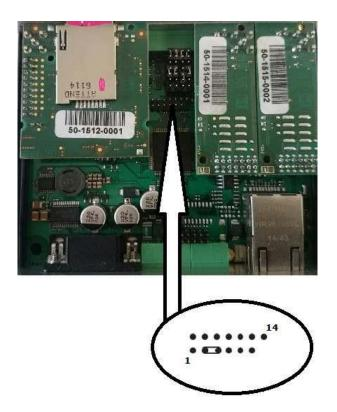
Connect the jumper as shown in the figure above. Interconnect pins 3 and 5. Now reconnect the power supply. Upon power up, the Flash memory is deleted and the factory default values are reset for all ports. Remember to remove the jumper to avoid deletion of the settings upon every start.
